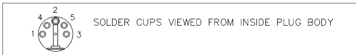
Fig. 2 DIN input connector pin identification - ZG units
