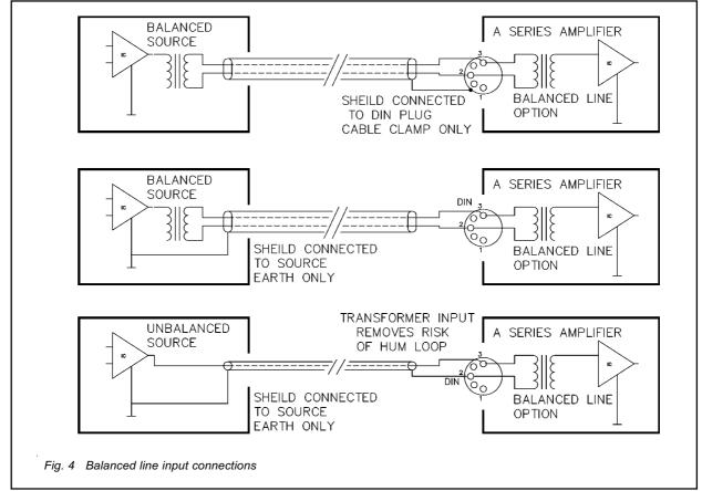
It would normally be appropriate to interconnect two pieces of equipment using twin-screened cable. The braiding should be earthed to one unit only. If the decision is made to use the Mustang power amplifier for earthing, then the cable clamp of the DIN plug may be used for the purpose, without the likelihood of a hum loop.
