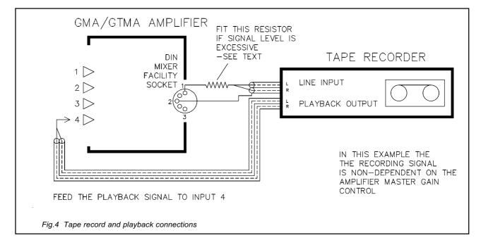
The manufacturer's handbook should be consulted to ensure that the recorder will accept signal levels of approximately 0.75V without distortion and that the recorder does not short out the signal recording connections when in the playback mode. In either case, insert a resistor of suitably high value in series with the recording lead. An experimental starting value would be 22k ohms. See Fig. 4
